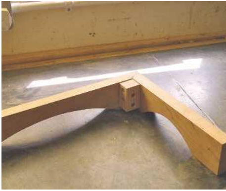
▲ Pic.7 The plinth has mitred joints, strengthened with blocks that were glued and screwed into the corners
